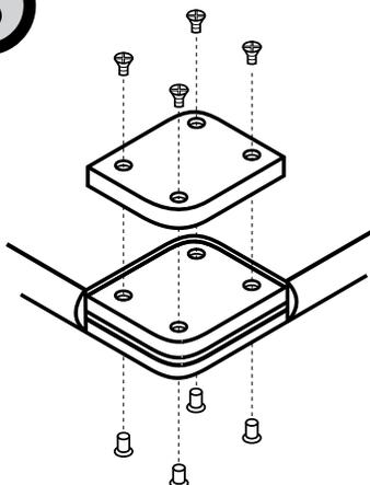
Using the Corner Saver as a template, mark and drill four 5/16" holes and countersink each hole. Fasten the Corner Saver with the four bolts and "T" nuts provided.
